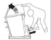
Repeat from the front and remove the front half of the polystyrene base.
